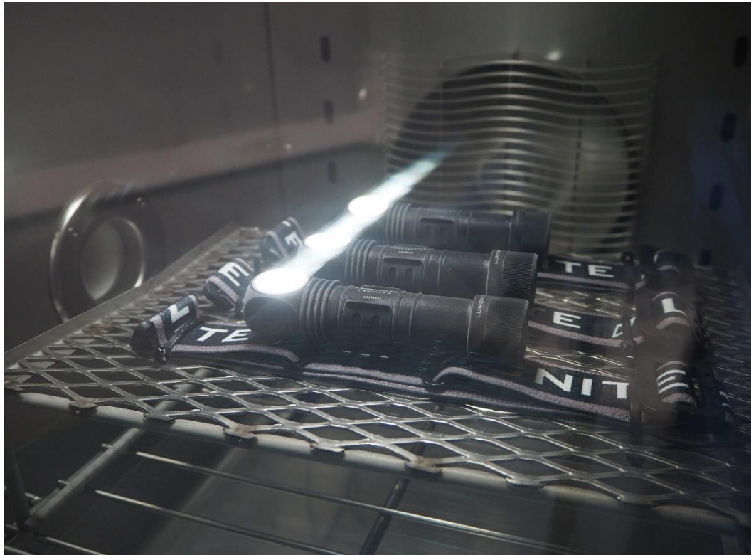
Picture 4. EUTs moved to elevated temperature chamber and frosting was seen on EUT's external surfaces
