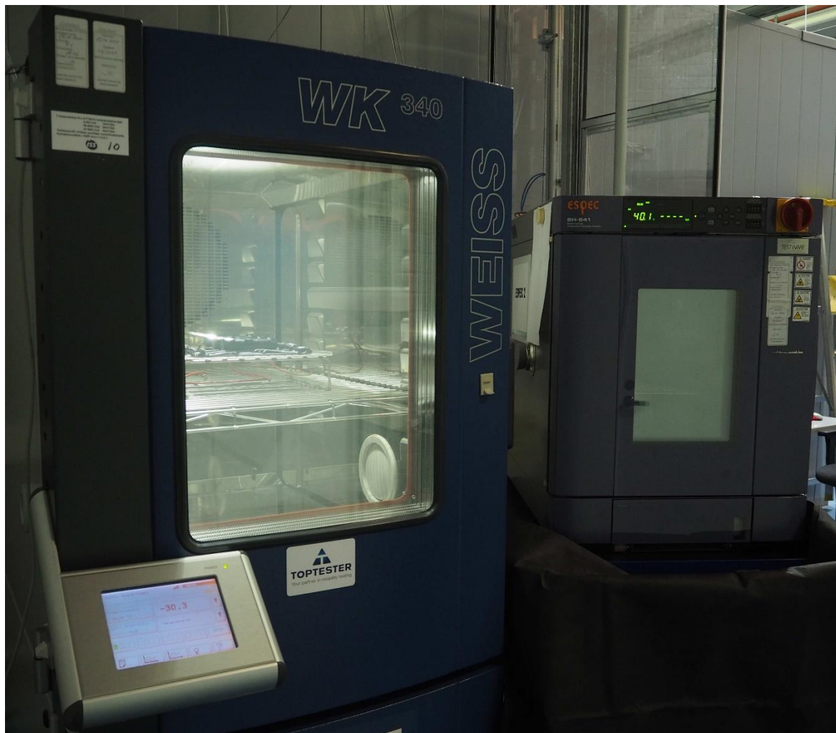
Picture 3. EUTs on cold temperature chamber and elevated temperature chamber
