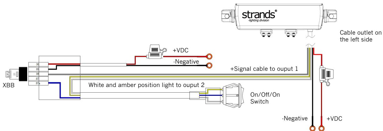
**Note:** The connection diagram shown is an example only, featuring the cable kit included in the package. This guide focuses on connecting an external switch and XBB. If you do not wish to connect with XBB, you may use other alternative methods. see connection diagram for 902001-03 on page nr 3.
