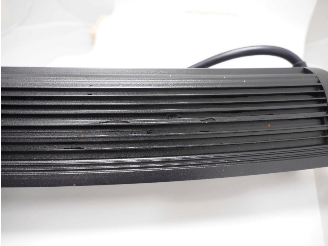
Figure 6. A small spot of corrosion was found from the EUT after test.
