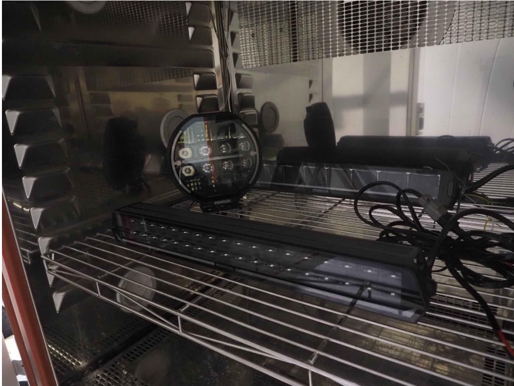
Figure 3. The EUT in environmental chamber.
