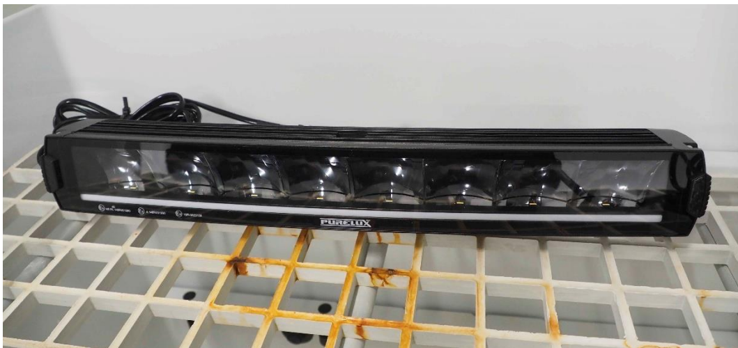
Figure 2. The EUT in salt mist chamber.
