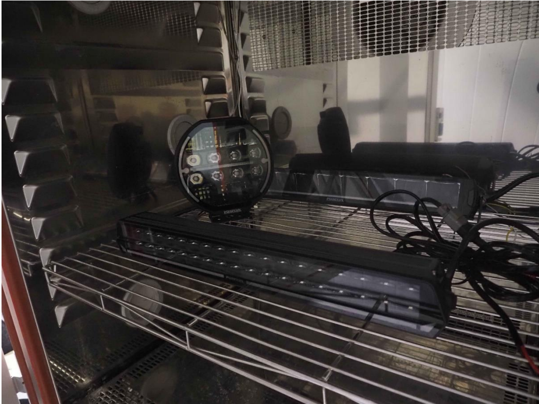
Figure 3. The EUT in environmental chamber.
