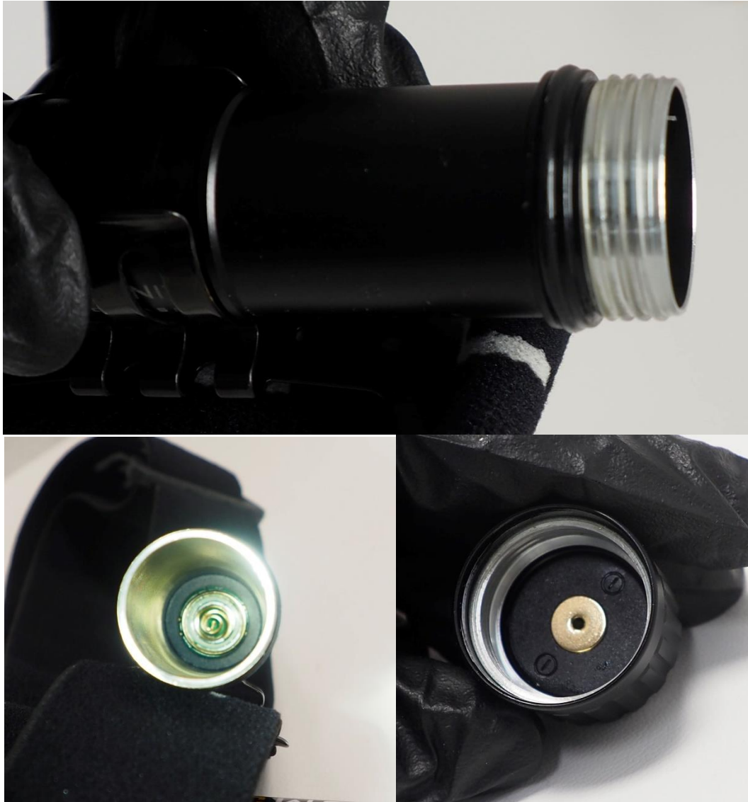
Figure 4. No salt penetration inside the battery box.
