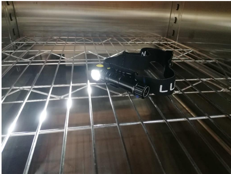
Figure 3. The EUT in cold test chamber.
