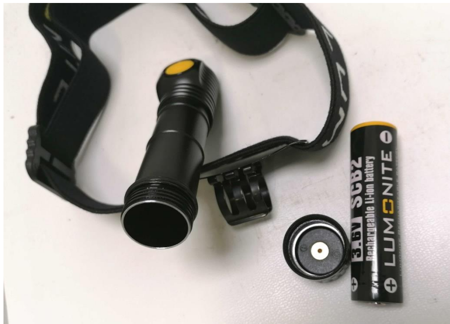
Figure 6. EUT after test. No physical damage was found after test.
