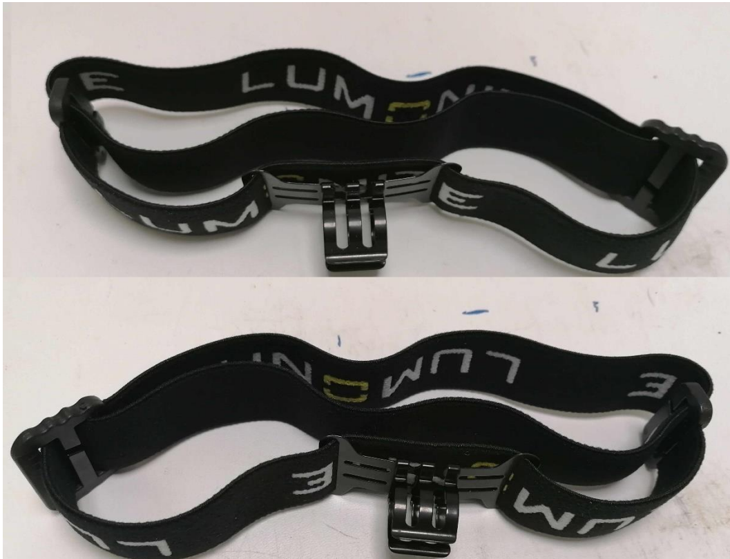
Figure 6. The headband after test. No physical damage was found after test.
