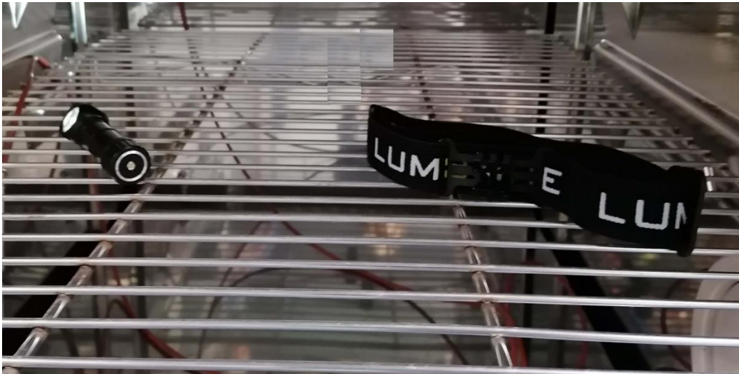
Figure 3. EUT in environmental chamber.
