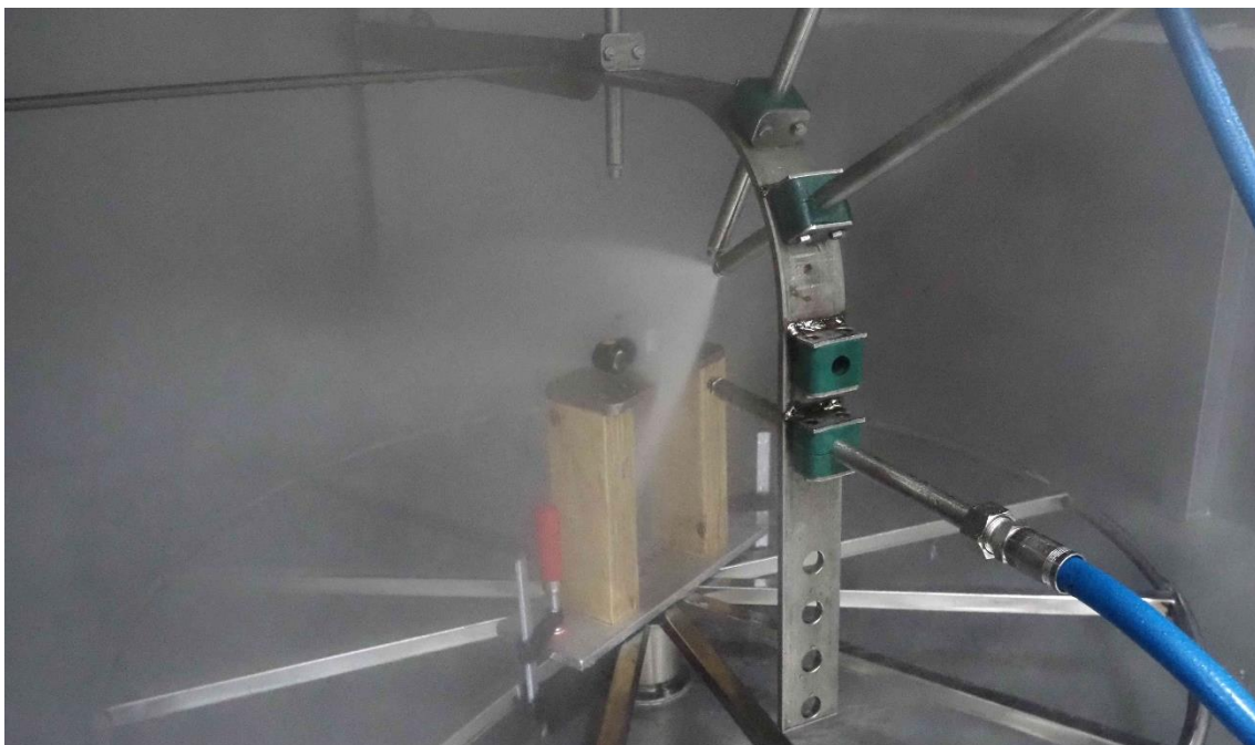
Figure 3. Ongoing IPX9 test.
