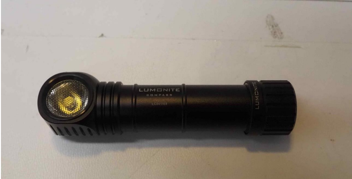
Figure 4. EUT after the test. No damage was detected.
