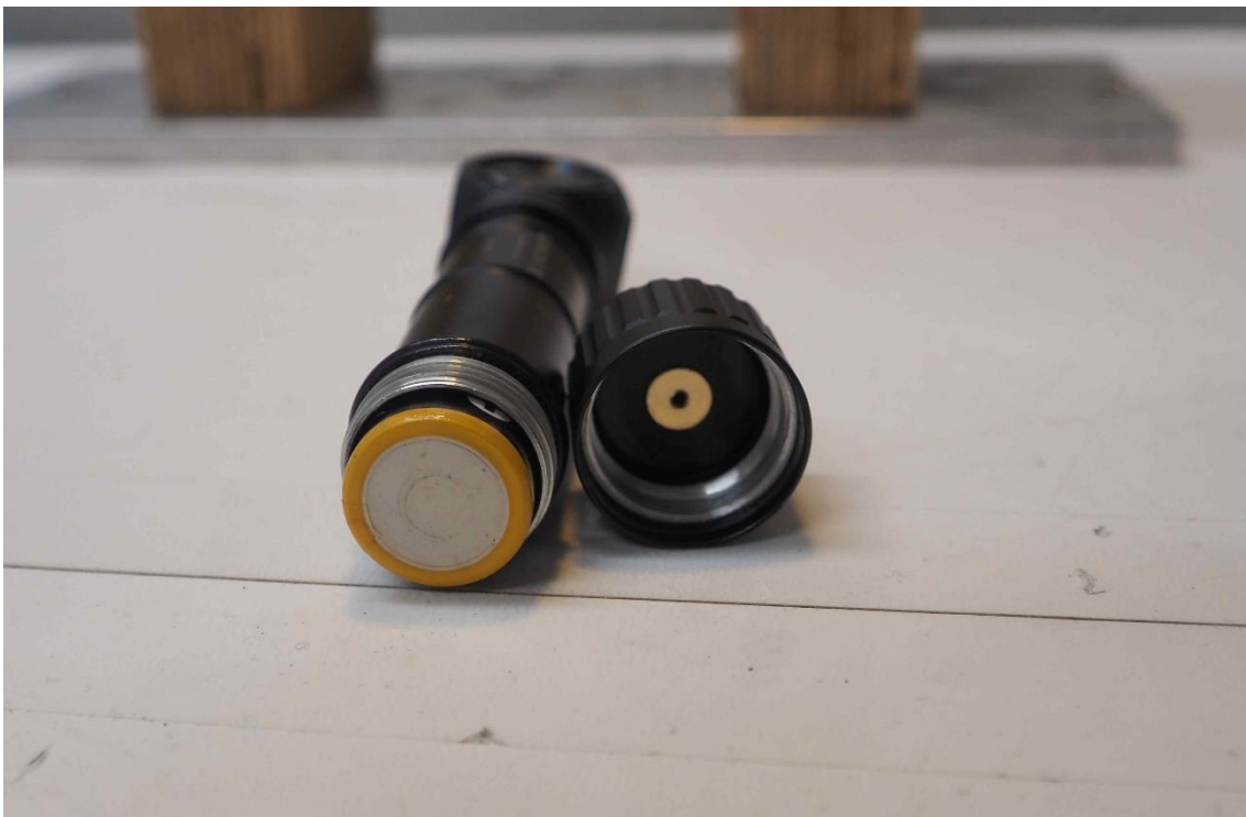
Figure 5. Battery case opened after test. No water was found inside.
