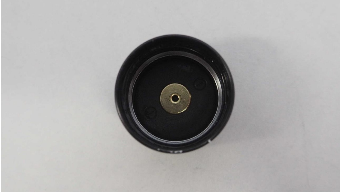
Figure 3. Battery case opened after test.
