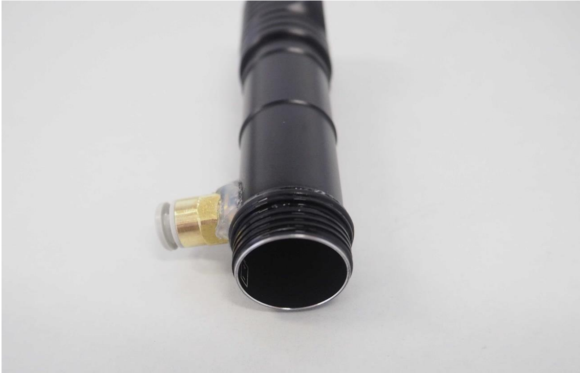
Figure 5. Battery case opened after test.
