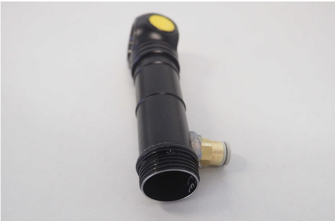
Figure 4. Battery case opened after test.
